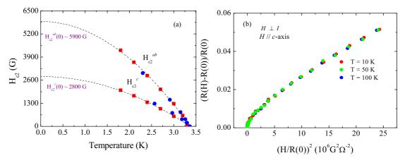
**Fig. 2** (a) Upper critical field  $H_{c2}$  for fields perpendicular and parallel to the *ab*-plane as a function of temperature. (•) and (•) were determined by R(H) at various T and R(T) at different H, respectively. (b) Normal-state transverse magnetoresistance ratio versus  $(H/R(0))^2$  plot at various temperatures. It is interesting to note that all the data collapse onto a universal curve.
