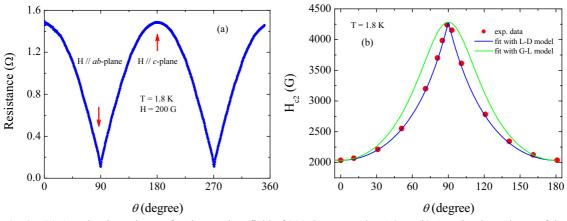
**Fig. 3** (a) Angular dependence of resistance in a field of 200 G measured at 1.8 K. (b) Angular dependence of the upper critical field  $H_{c2}$  at 1.8 K. The solid points are experimental data, whereas the blue and green curves are fitting to L-D and G-L model, respectively.
